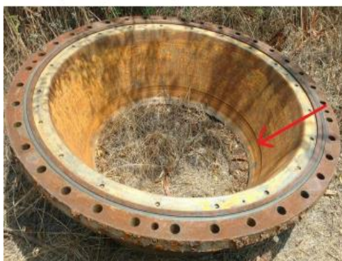
Rubbing of Impeller casing observed
