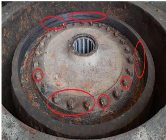
Pump casing bolt complete wear out, pitting on casing wear ring
