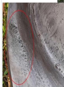
Close view of Pitting/cavitation on impeller blades
