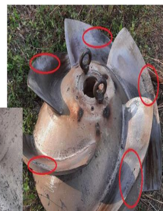
Pitting/cavitation on impeller
