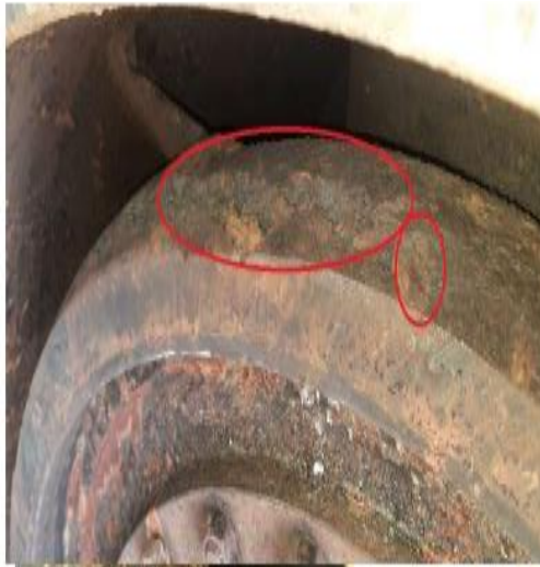
Pump casing bolt complete wear out, pitting on casing wear ring
