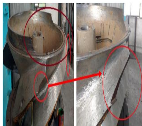
Damaged Impeller, Impeller ring along with impeller vanes rubbing observed.
