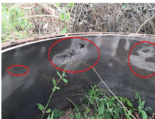
Through hole to impeller casing and liner assembly
