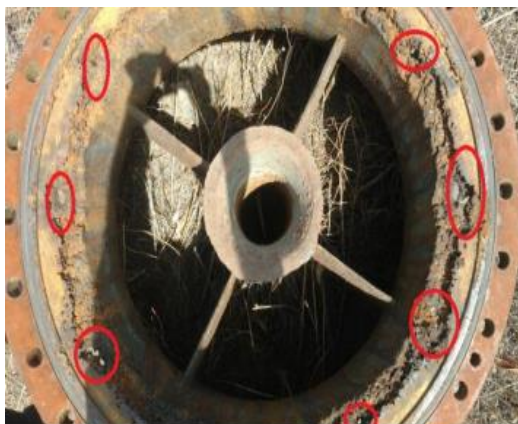
Rubbing of Impeller casing observed
